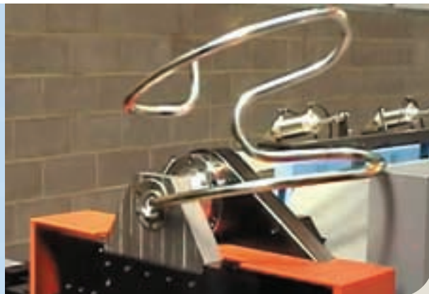
Stainless steel tube bending for marine and architectural fittings, a typical machine tool application using rotary vane actuators with vane seals.
