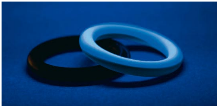
Uncoated and coated seal under UV-light
